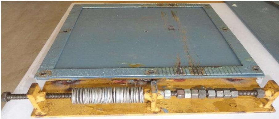
**FIGURE 1.** In-house developed mold assembly.
