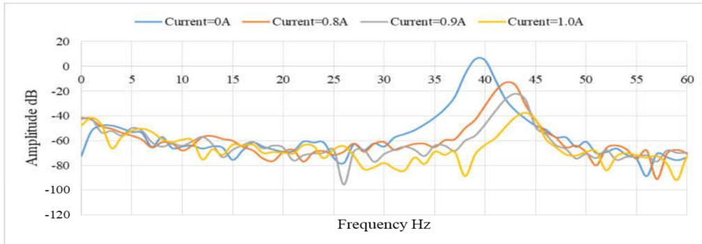
**FIGURE 4.** Frequency response of SMAHC beam with single wire.
