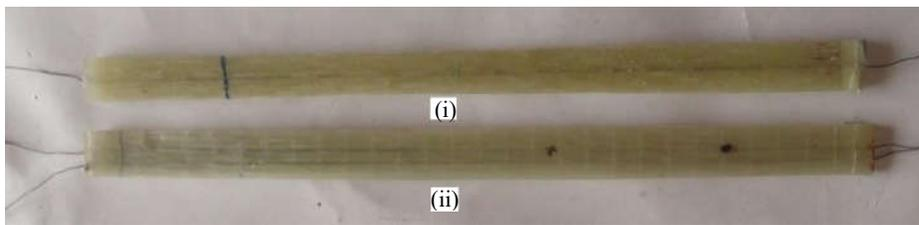
**FIGURE 2.** Shape memory alloy hybrid composite beams: (i) single wire and (ii) two wire.
