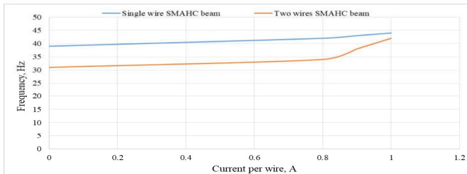
**FIGURE 5.** Fundamental natural frequency vs. current plot of single and two wire SMAHC beams.
