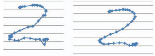
Fig. 5: Before and After Trajectory Smoothing of Gesture Path
