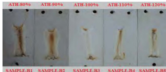
Fig. 2. Photograph of B1 to B5 subjected to IPTET+UV
