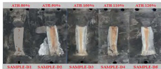
Fig. 4. Photograph of D1 to D5 subjected to IPTET+HC+UV
