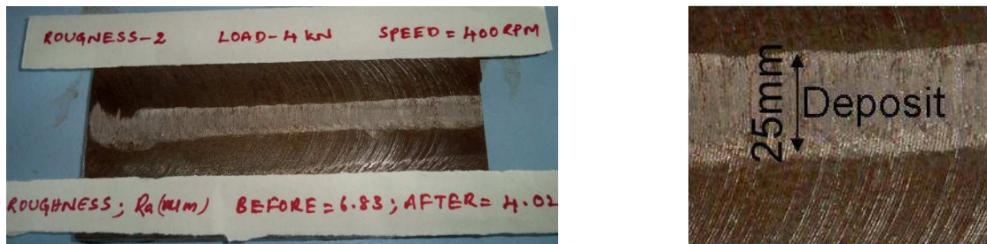
Fig. 2 Shows macroview of a sample with good deposition (S4). On the right side enlarged view of the deposition is given. We see that deposition is continuous and width is uniform.
