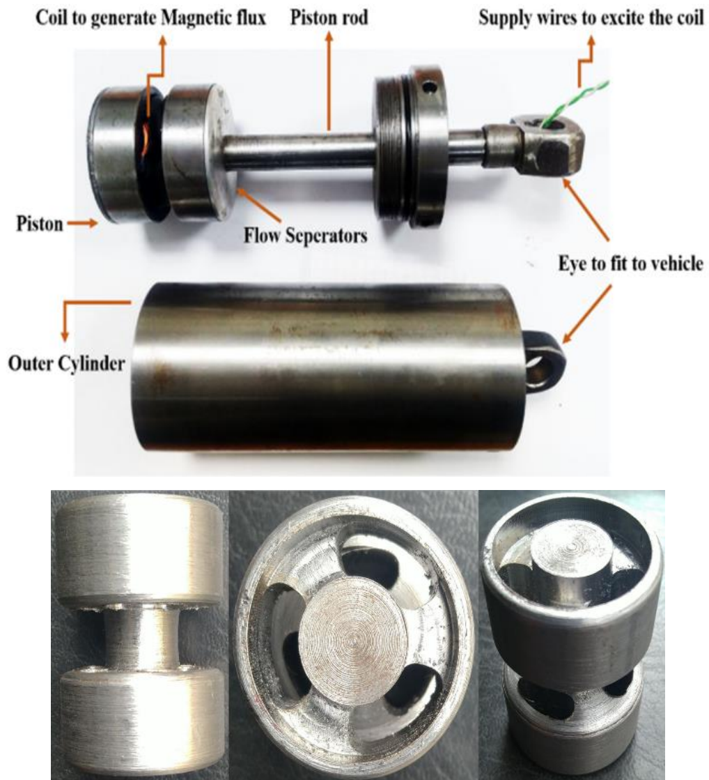
Figure 6.5 Developed MR damper with detailed view of Hybrid Radial Flux Piston
