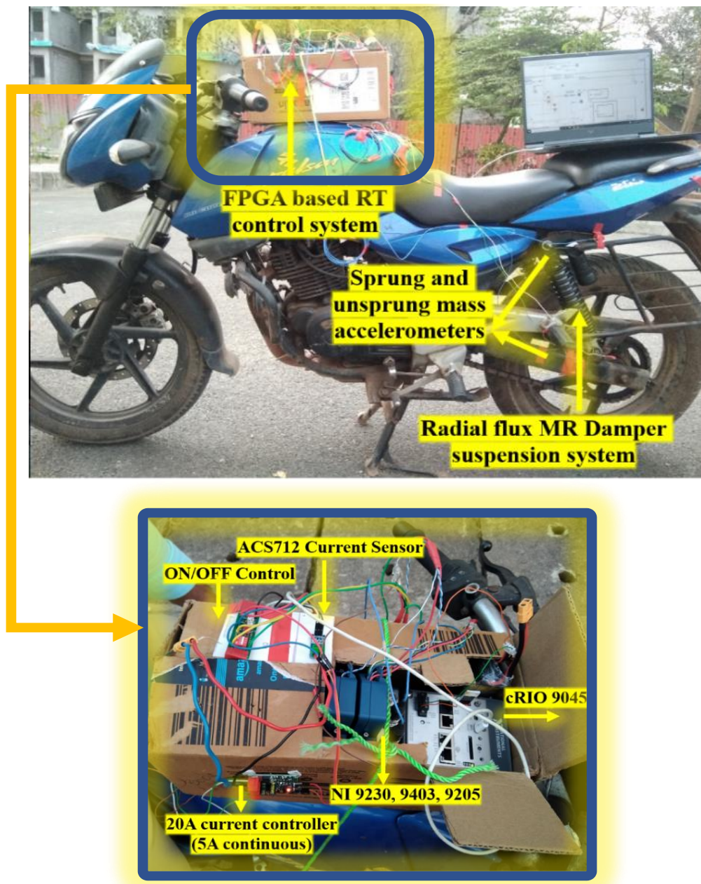
Figure 4.19 Two-wheeler RT experimentation test setup along with the controller
