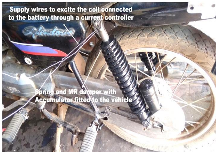
Figure 2.7 MR damper used two-wheeler vehicle Devikiran et al. (2021 )
