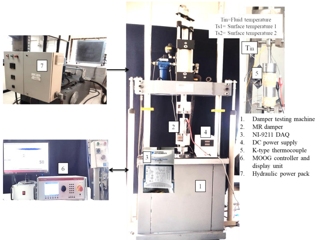
Figure 4.8 DAQ and controller setting for temperature characterisation
