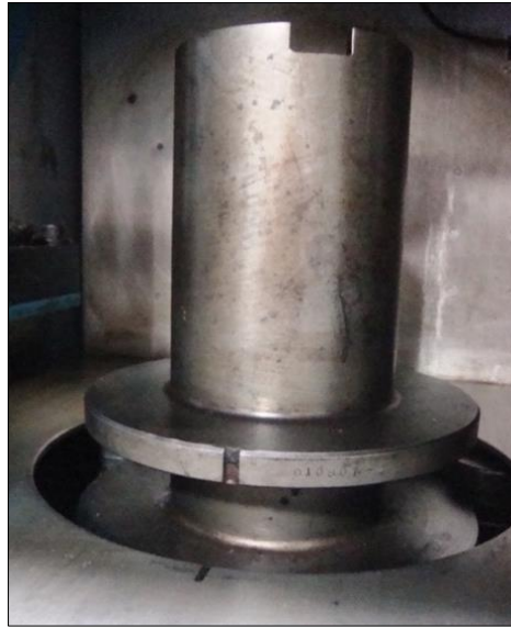
Fig. 3.14 SGC mould of 100 mm diameter
