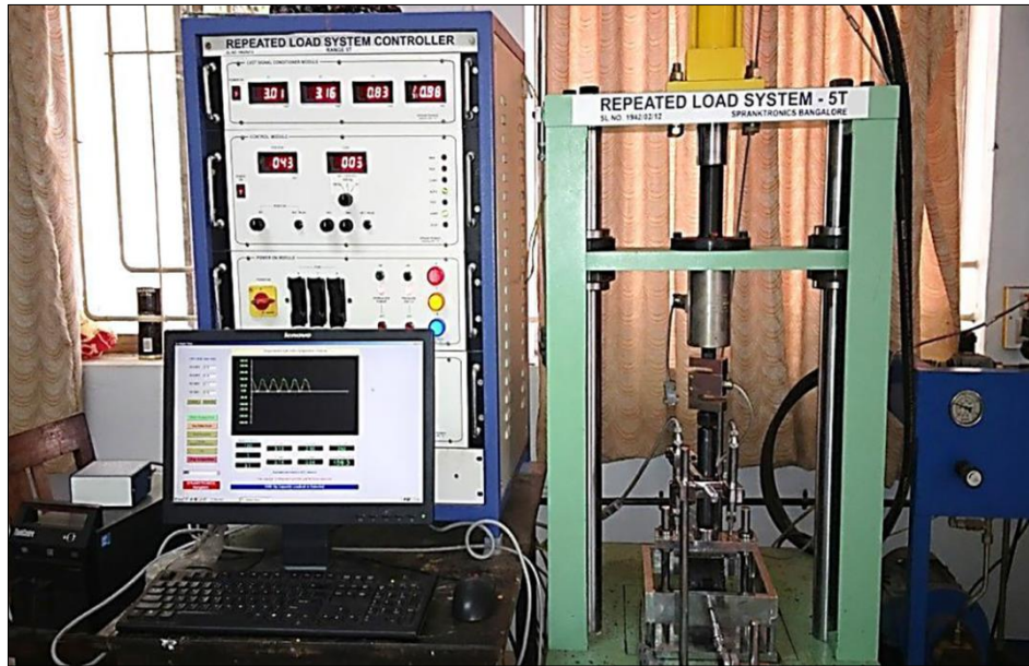
Fig. 3.19 Repeated Load Testing (RLT) Device
