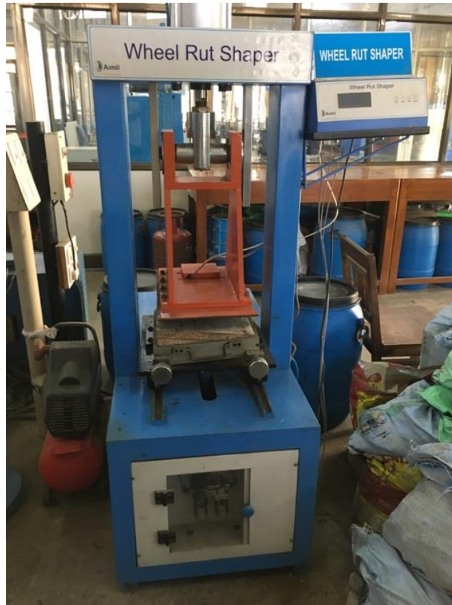
Fig. 3.18 Wheel Rut Shaper
