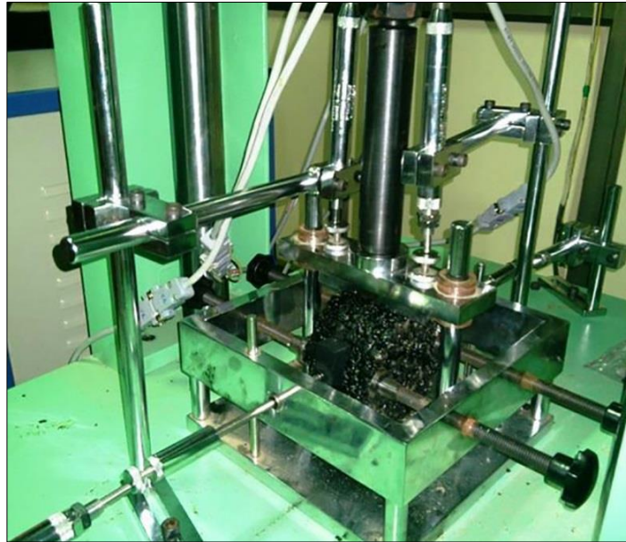
Fig. 3.20 Specimen arrangement in RLT device
