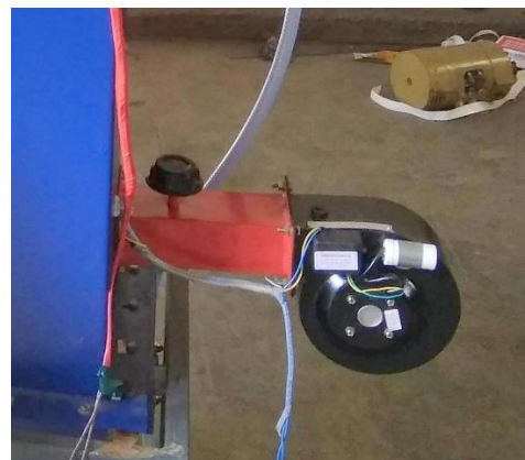
(h) Air Blower
