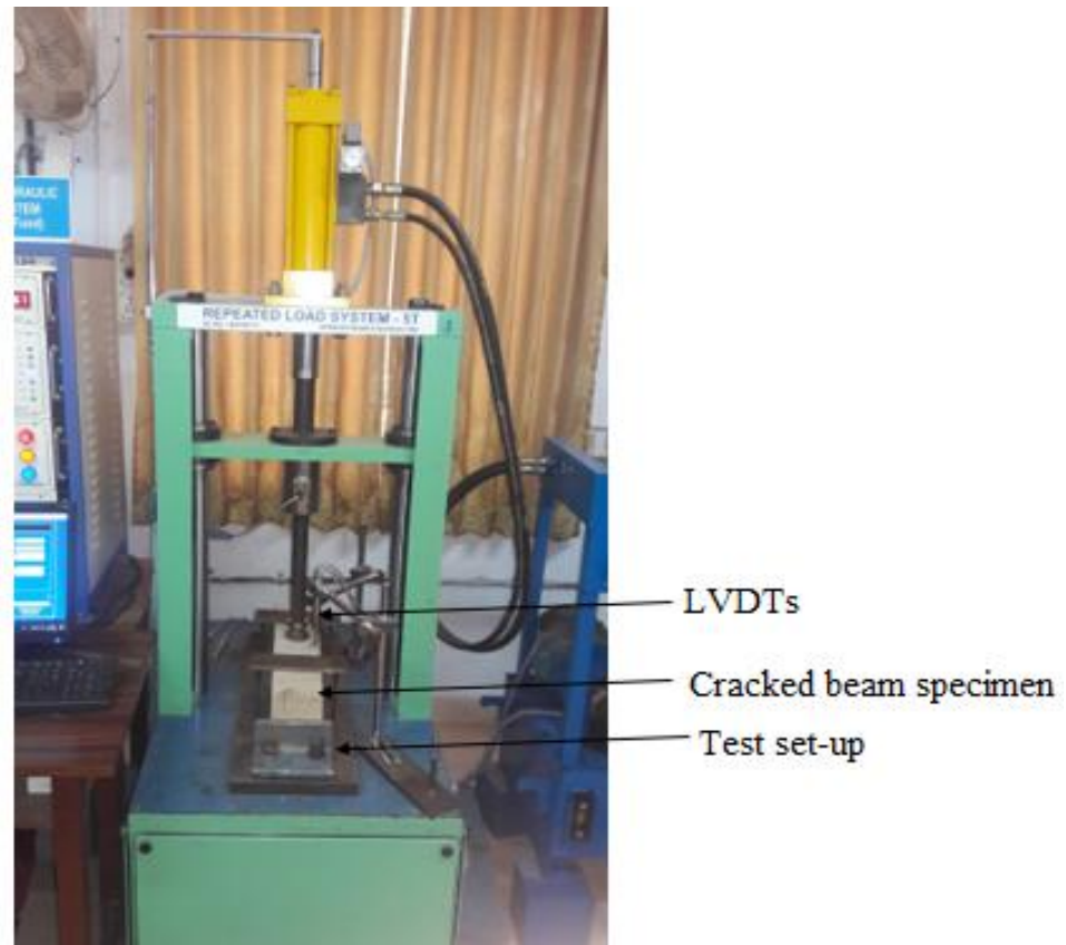
Figure 3.14 Small-scale test setup along with specimen
