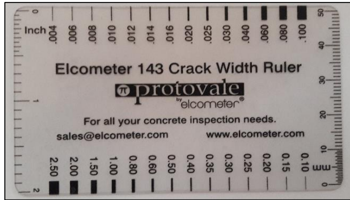
Figure 3.15 Crack width ruler used in the present study
