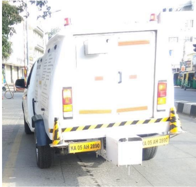
Figure 3.16 KUAB 70 vehicle-mounted falling weight deflectometer (FWD)
