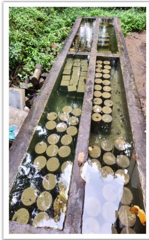
Figure. 3.5 Curing of concrete specimens in freshwater
