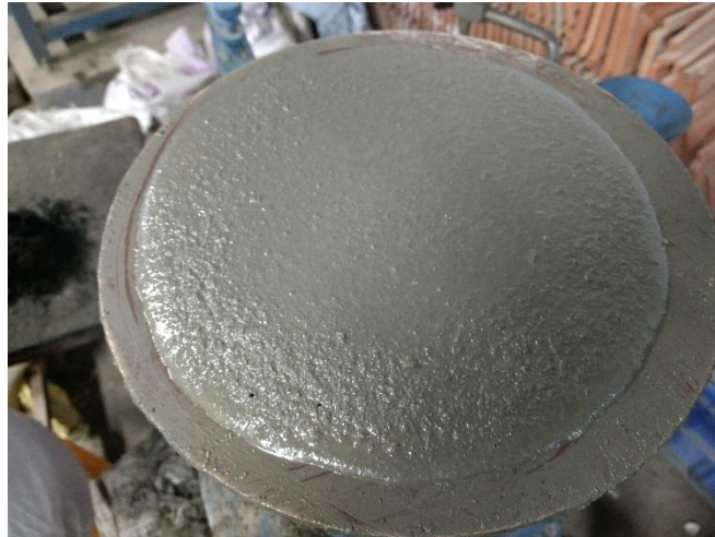
Figure 3.4 Flow table test of mortars
