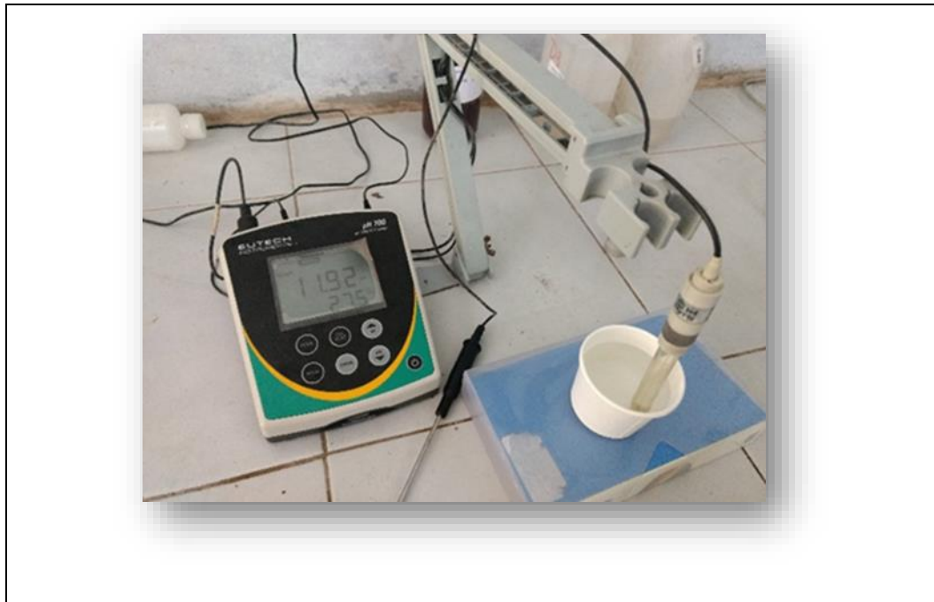
Figure. 3.10 pH of concrete
