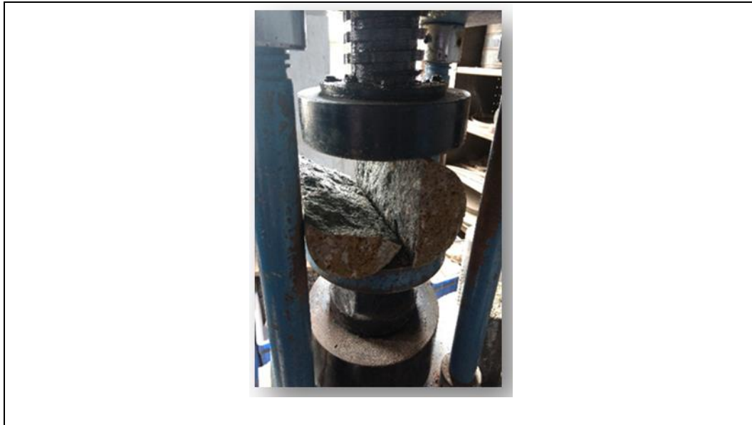
Figure. 3.8 Splitting tensile strength of the concrete
