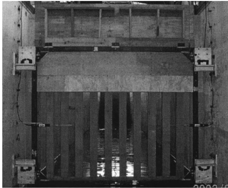
Fig. 2.9 Lee side view of pile supported vertical wall breakwater (Suh et al. 2006)
