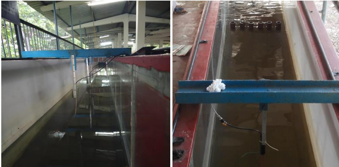
Fig. 3.36 View of wave flume with wave probes for data acquisition
