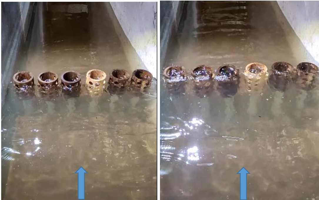
a) Wave crest approaching pile head b) Wave crest plunging into hollow portion
