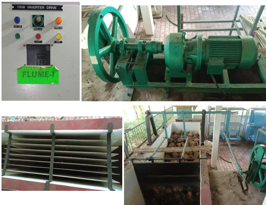
Fig. 3.37 Wave generation system (clockwise from top left: inverter drive, motor, flap type wave paddle and wave filter)
