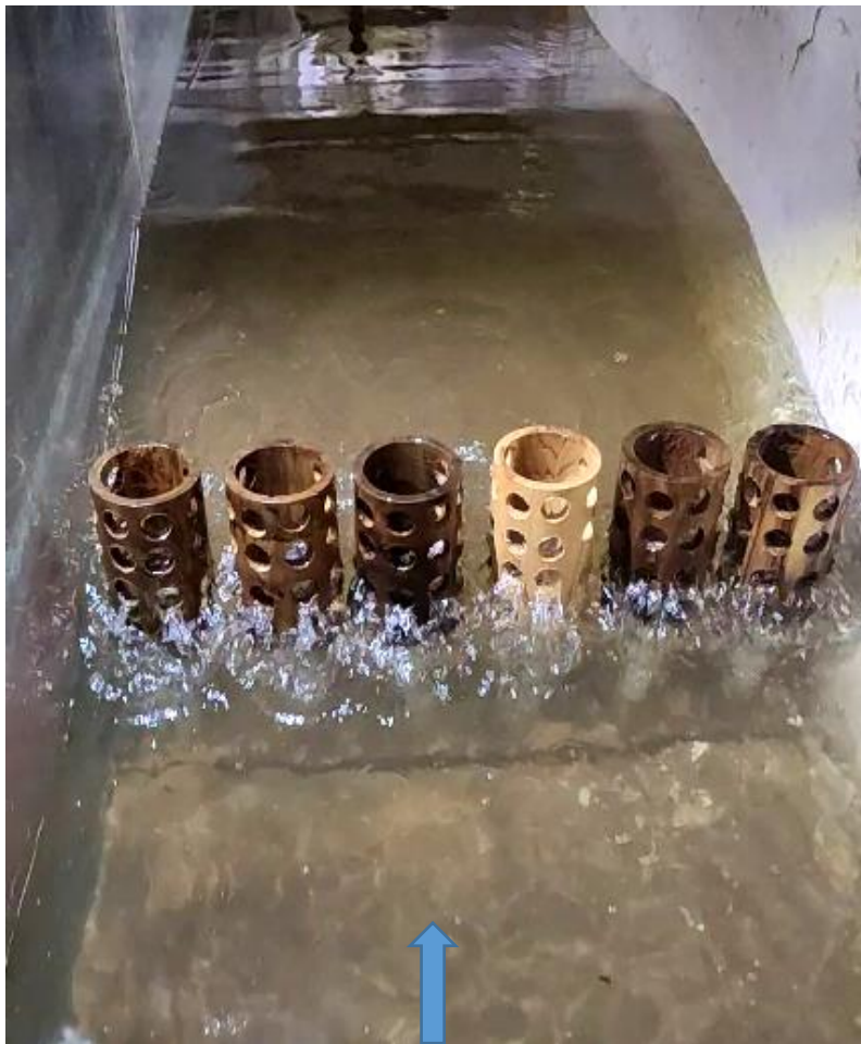
Fig. 3.31 View of water flowing back (towards seaside) under wave trough from the perforated of enlarged pile head
