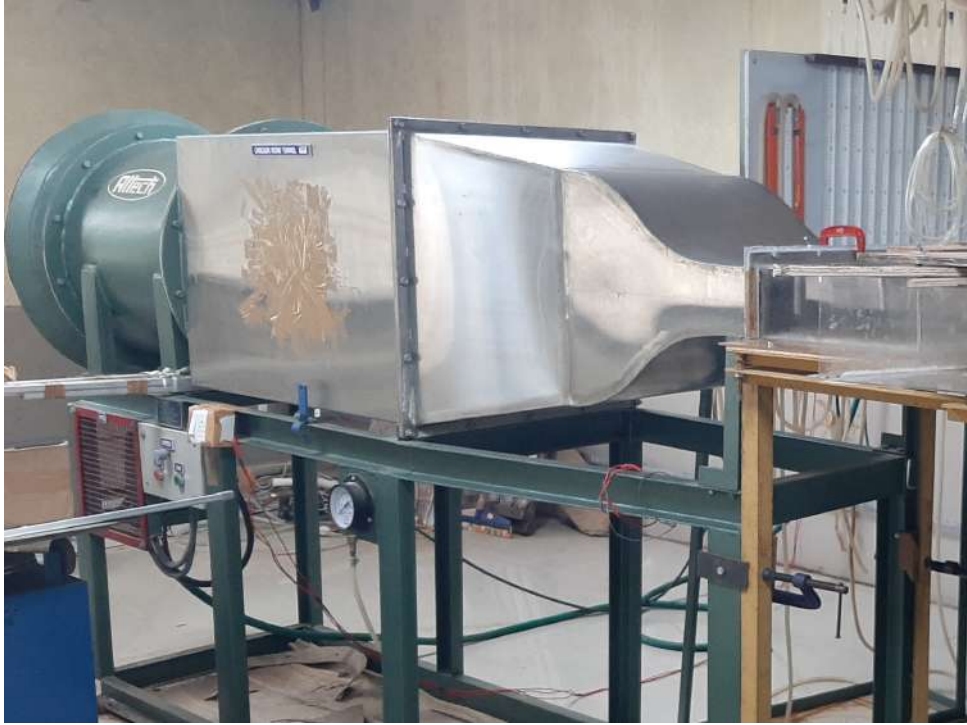
Figure 3.1: Blowing type subsonic cascade wind tunnel.
