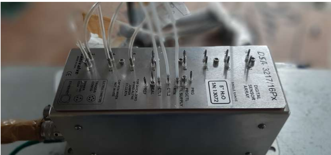
Figure 3.8: Digital sensor array - 16 channel pressure transducer (Scanivalve DSA3217).
