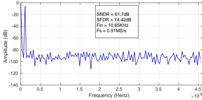
Figure 5.14: FFT spectrum of 10 bit ADC for an input frequency of 10.65 KHz
