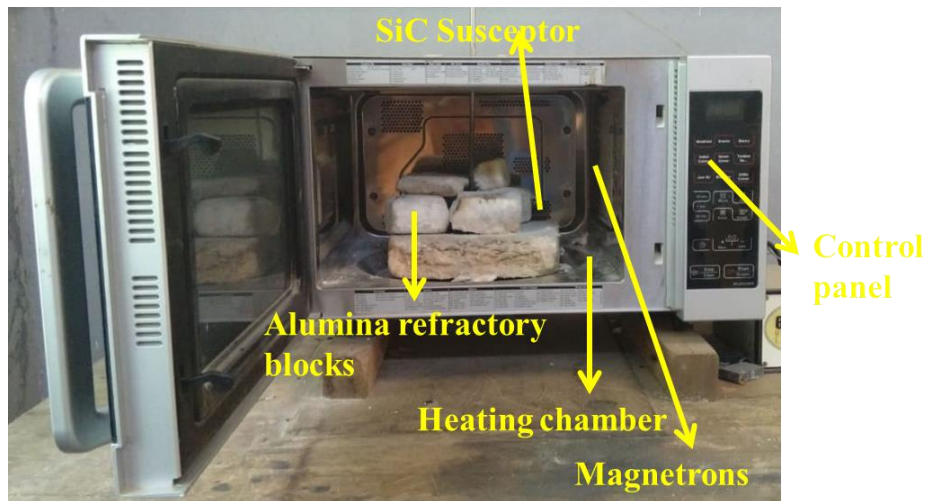
Figure 3.4 Domestic microwave oven set up
