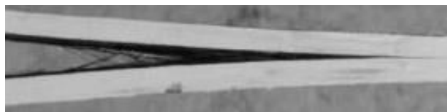
Fig. 1.4 Uni-directional fiber bridging (Robinson and song 1992)
