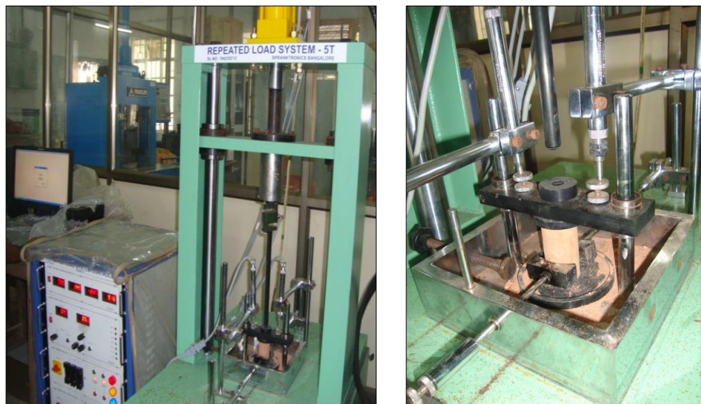
Fig. 7.6 Fatigue testing machine and sample arrangement
