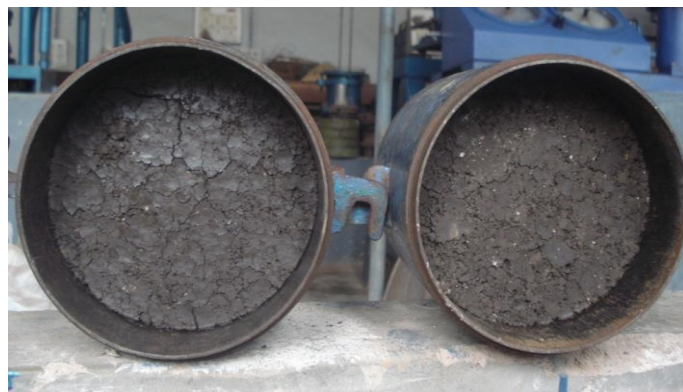
Fig. 5.5 CBR treated samples after seven days open air curing
