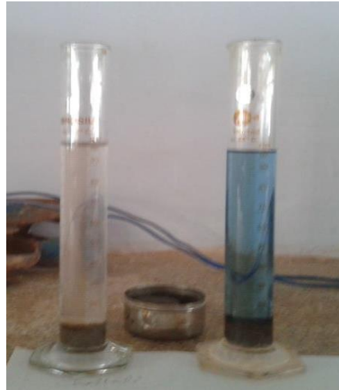
Fig. 3.4 Set up for FSI
