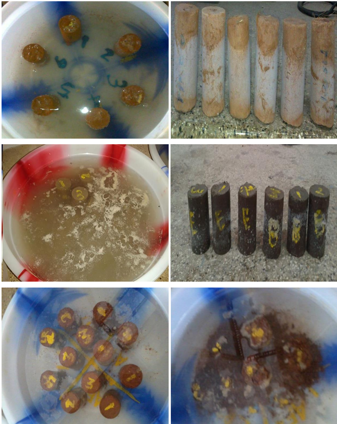
Fig. 6.1 Durability specimens during wet-dry and thawing cycles
