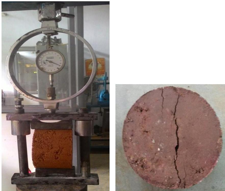
Fig. 7.1 IDT strength set up and failed specimen
