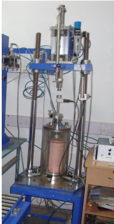
Fig. 3.5 Tri axial set up
