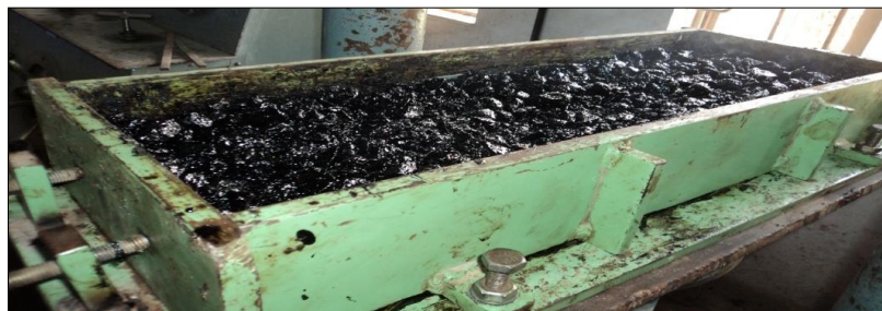
Fig. 3.14 Placing of Mix for Preparation of Rutting Sample
