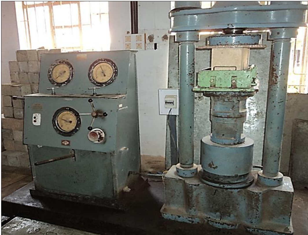
Fig. 3.15 Compaction of Rutting Slab
