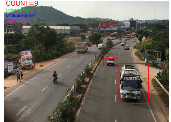
(b) 860 th frame of video 1.mp4. Total no of vehicles passed are displayed at the top corner. Traffic count is also classified as small (LOWCOUNT), medium (MEDIUMCOUNT) and large (HIGHCOUNT) categories. Vehicles in the tracked state are shown using red bounding box.
