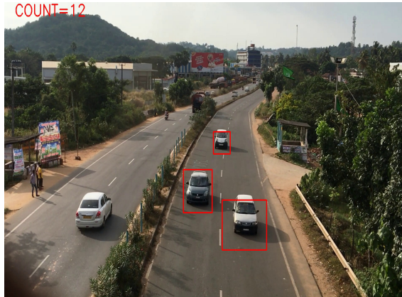
(a) 575 th frame of video 2.mp4. Total no of vehicles passed are displayed at the top corner. Vehicles under tracked state are shown using red bounding box.
