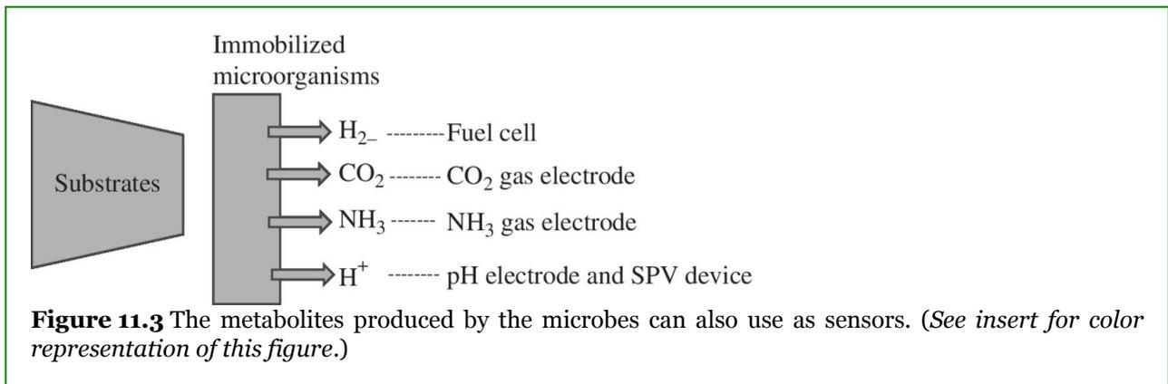
The transducers for H<sub>2</sub> detection have been fuel cell type, CO<sub>2</sub> electrodes, NH<sub>3</sub> electrodes, or pH electrodes (including ion-sensitive field-effect transistors (ISFETs)). Most of these sensors are based on potentiometry. Though they have a large measurable range, there have a limitation of lower detection limits
