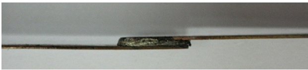
Fig. 4 Side view of Cu/solder/Cu lap solder joint
