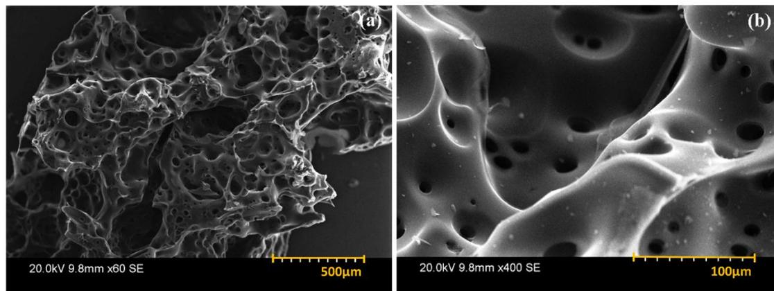
**Figure 5:** (a) Low magnification and (b) high magnification of Scanning electron micrograph of CO<sub>2</sub> activated carbon at 900 °C for 8 hours.
