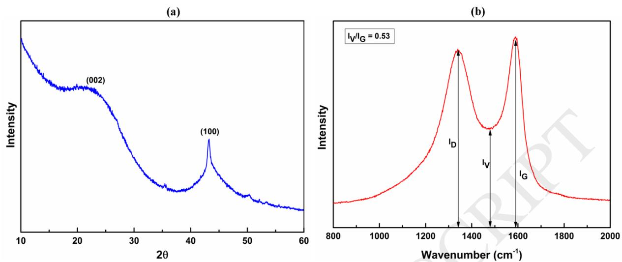
**Figure 6:** (a) XRD and (b) Raman spectra of activated carbon from waste CD activated at 900  $^{\circ}\text{C}$  for 8 hours.
