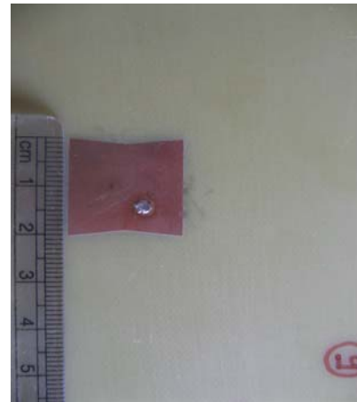
Fig 3(b) Designed square patch antenna with identical notch angles
