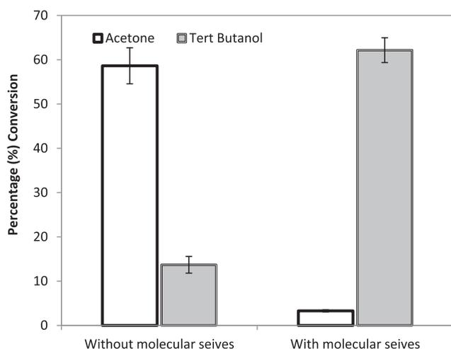
**Fig. 7.** Effect of addition of molecular sieves on the lipase-catalysed esterification of rutin with decanoic acid for 96 h with 15 mg/mL enzyme load and 1:4 rutin: fatty acid molar ratio at 55 °C and 150 rpm. Bars represent standard deviation ( $n = 2$ ).
