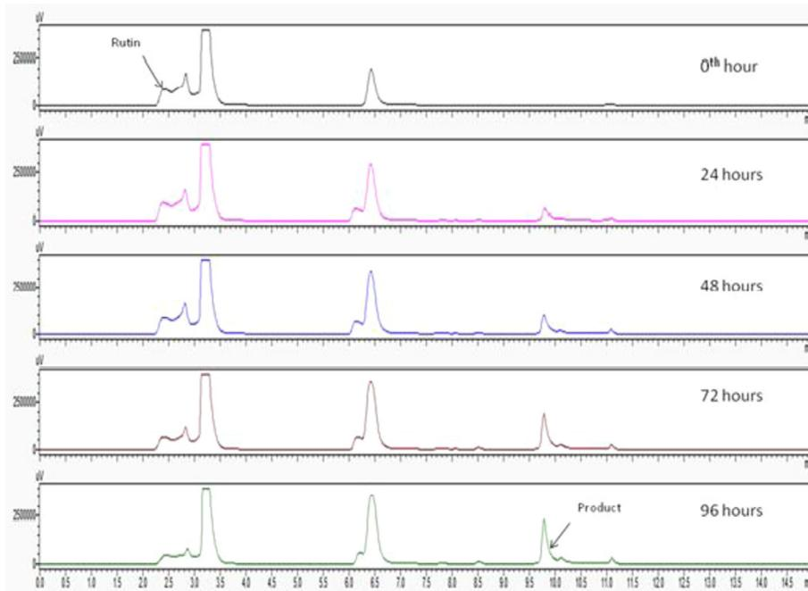
**Fig. 2.** HPLC chromatograms at 254 nm of reaction mixture of lipase catalysed esterification of rutin and decanoic acid over a period of 96 h. Peaks were identified as follows: rutin (2.8 min) and rutin decanoic ester (9.7 min).
