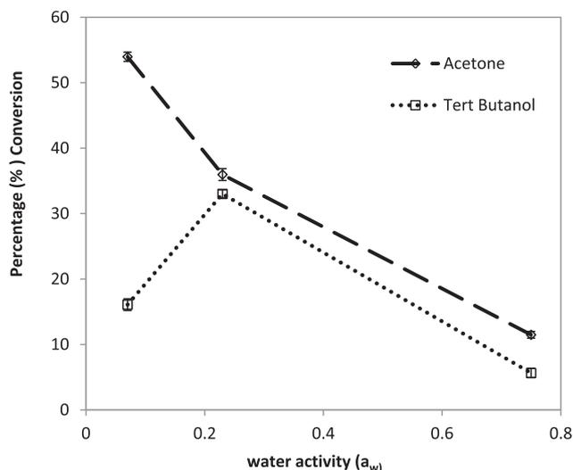
**Fig. 6.** Effect of water activity on the lipase-catalysed esterification of rutin with decanoic acid for 96 h with 15 mg/mL enzyme load and 1:4 rutin: fatty acid molar ratio at 55 °C and 150 rpm. Bars represent standard deviation ( $n = 2$ ).
