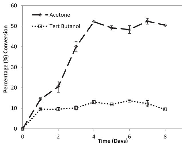
**Fig. 4.** Lipase-catalysed esterification of rutin with decanoic acid over a period of eight days at 55 °C, 150 rpm with 15 mg/mL enzyme load and 1:4 fatty acid:rutin molar ratio without setting water activity. Bars represent standard deviation (n = 2).
