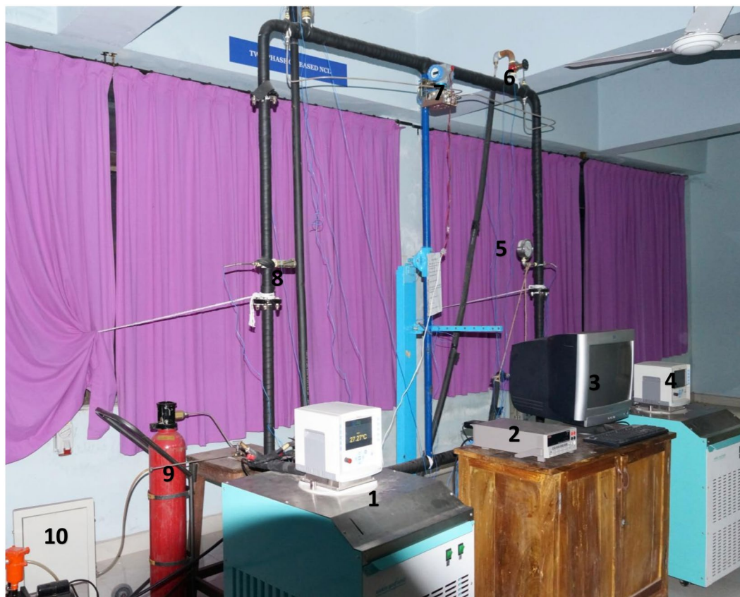
Figure 2. Experimental setup. (1) Thermostatic bath- 1(HHX), (2) DAQ, (3) Computer to read DAQ Data, (4) Thermostatic bath –2(CHX), (5) Pressure Gauge, (6) Rotameter, (7) Differential Pressure Transducer, (8) Safety Valve, (9) CO 2 cylinder, (10) Vacuum pump.
