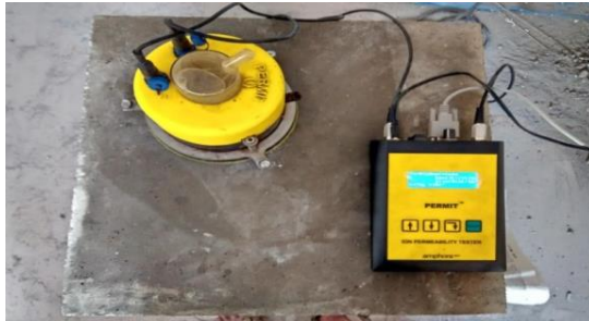
Fig. 8 (b) Permit ion permeability test on PS ball concrete sample
