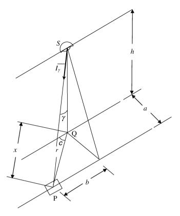
Figure 2. Illuminance on a horizontal plane.
