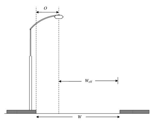
Figure 1. Effective road width ( $W_{eff}$ ) equal to actual width (W) minus luminaire overhang (O).
