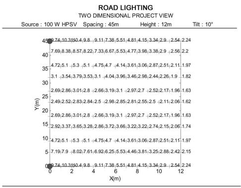
Emin: 1.62 Emax: 10.4 Eave: 4.0881 Emin/Eave: 0.39627 Emin/Emax: 0.15577 Figure 5. Spot illuminance levels with 100 W HPSV lamps at 12 m pole height.
