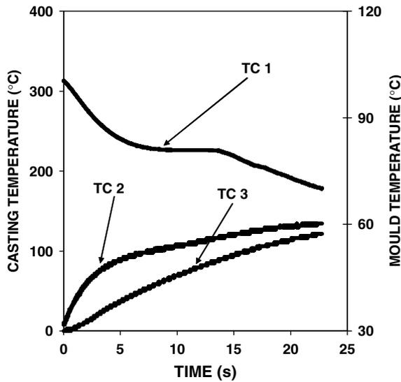
Fig. 5. Typical casting and mould thermal history during solidification of solder alloy (Sn–0.7Cu).
