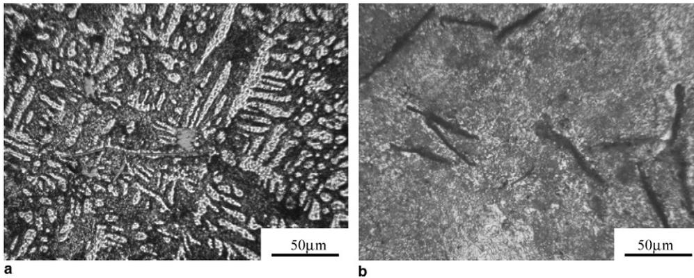
Fig. 9. Photomicrographs of: (a) Sn-3.5Ag solder and (b) Sn-9Zn solder alloys cast in copper mould.
