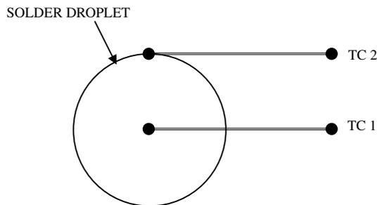
Fig. 1. Schematic sketch of solder droplet instrumented with virtual thermocouples.
