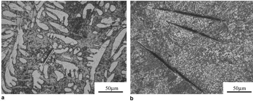
Fig. 8. Photomicrographs of: (a) Sn-3.5Ag solder and (b) Sn-9Zn solder alloys cast in stainless steel mould.
