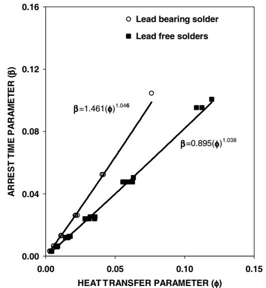
Fig. 4. Variation of arrest time parameter ( $\beta$ ) with heat transfer parameter ( $\phi$ ) for solder alloys.
