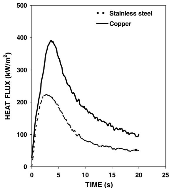
Fig. 6. Variation of heat flux with time during solidification of Sn–37Pb solder alloy.
