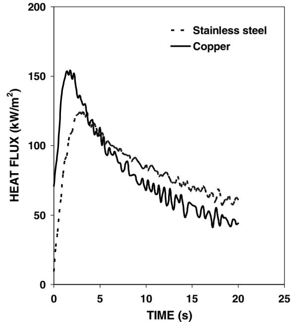
Fig. 7. Variation of heat flux with time during solidification of Sn–3.5Ag solder alloy.
