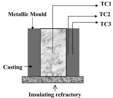
Fig. 2. Schematic sketch of experimental set up for solidification.
