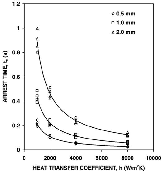
Fig. 3. Variation of arrest time ( $t_s$ ) with heat transfer coefficient ( $h$ ) for various solder droplet sizes.
