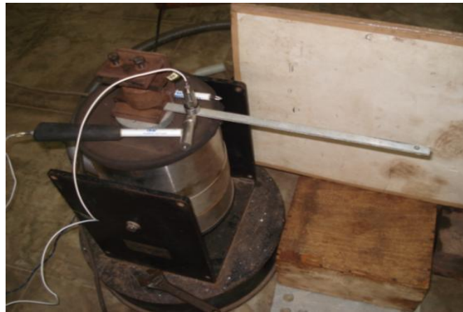
Plate 4.1 Cantilever fixed on shaker
