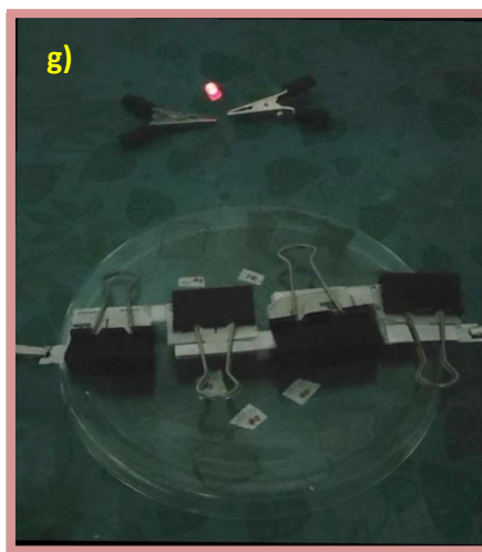
Figure 4.7: a) Nyquist plot and Cyclic stability of b) 5 wt% AC-P 2 W 18 , c) 10 wt% AC-P 2 W 18 and d) 15 wt% AC-P 2 W 18 and LED images of e) blue f) Yellow and f) Red light using the 5 wt% Ac-P 2 W 18 Electrode material.
