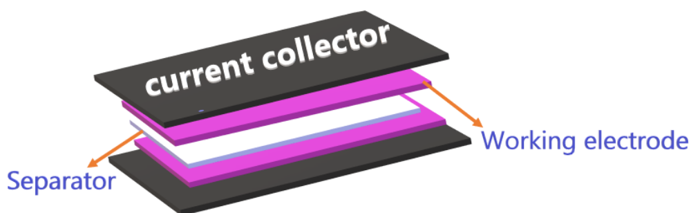
Figure 2.6: Schematic representation of two electrode configuration setups.
