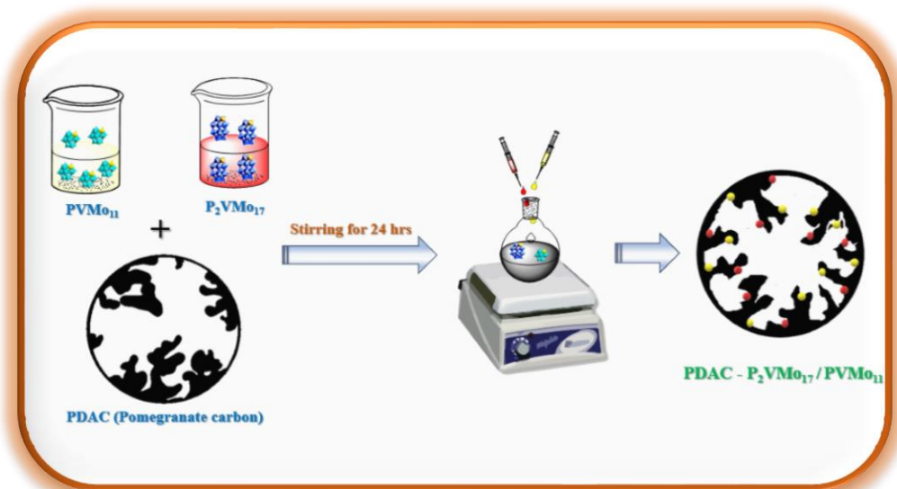
Figure 2.5: Schematic representation of infused Wells-Dawson and Keggin Polyoxometalates in pomegranate-derived activated carbon.
