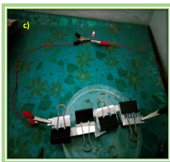
Figure 3.10: The cyclic stability response of (a) OPAC and (b) OPAC-PMA for 4000 cycles at a fixed current density of 6 \text{ A g}^{-1} and (c) The fabricated supercapacitors are energizing red light-emitting diodes.
