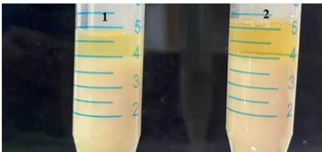
Figure 5.48b Chitin substrates after treatment with purified chitinase for 24 hours (1 and 2 – chitin powder and flakes, respectively)
