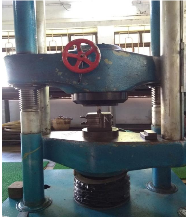
Figure 3.6: Hydraulic press with MDF set up.
