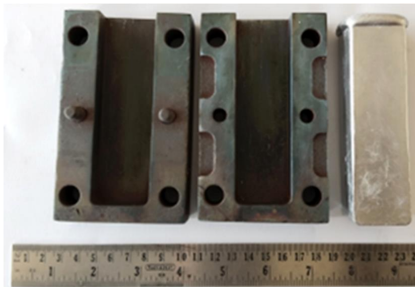
Figure 3.2: Casting die with cast sample.
