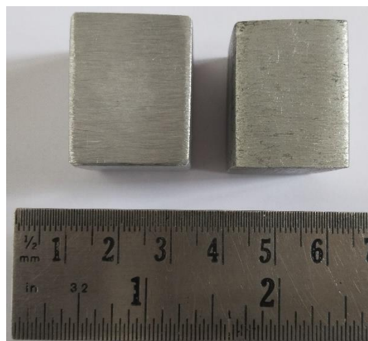
Figure 3.3: Al-7.3Si and Al-12.1Si samples for MDF Processing.
