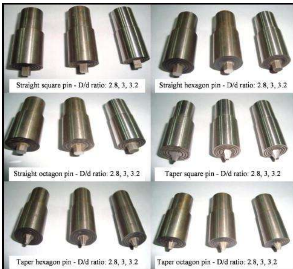
Figure 2.22 FSW tools with different pin profiles (Vijay and Murugan 2010)
