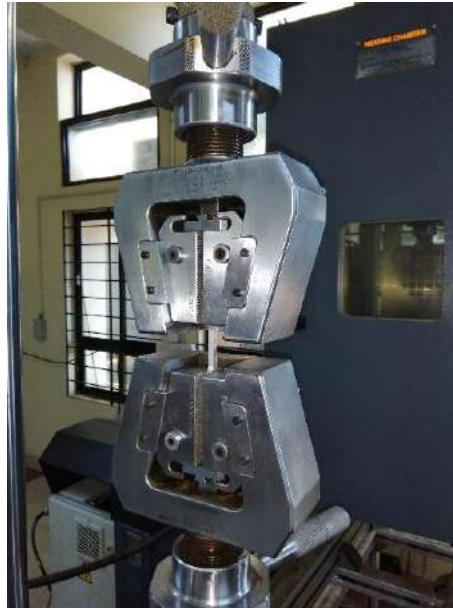
Figure 3.14 Fixture setup for tensile test on the universal testing machine
