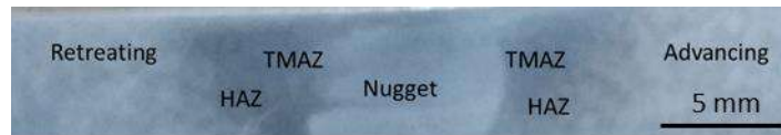
Figure 3.12 Image of composite joint FS welded using CSTC tool, showing advancing and retreating side, Nugget zone, TMAZ, HAZ.
