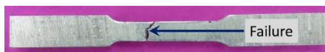
Figure 4.31 Fractured tensile specimen of FS Welded composite joint tested in the weld direction.
