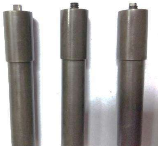
Figure 3.8 Fabricated and heat treated Friction stir welding tool with a) Threaded cylindrical pin, b) Square pin, and c) Combination of Square and Threaded cylindrical pin
