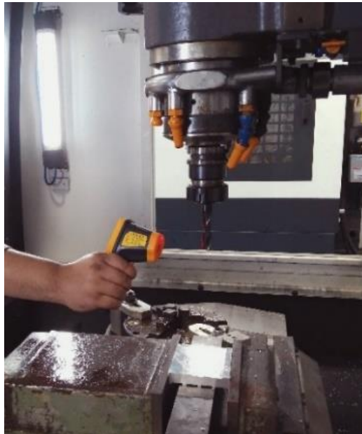
Figure 3.12 Cutting tool tip temperature measurement
