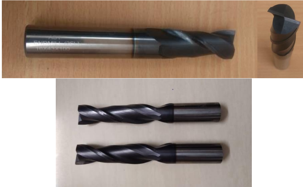
Figure 3.7 Solid carbide end mill cutter with two flutes
