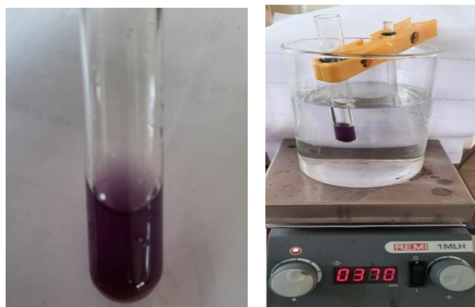
Fig. 3.3 Ninhydrin test of L-Leucine functionalized onto NFO
