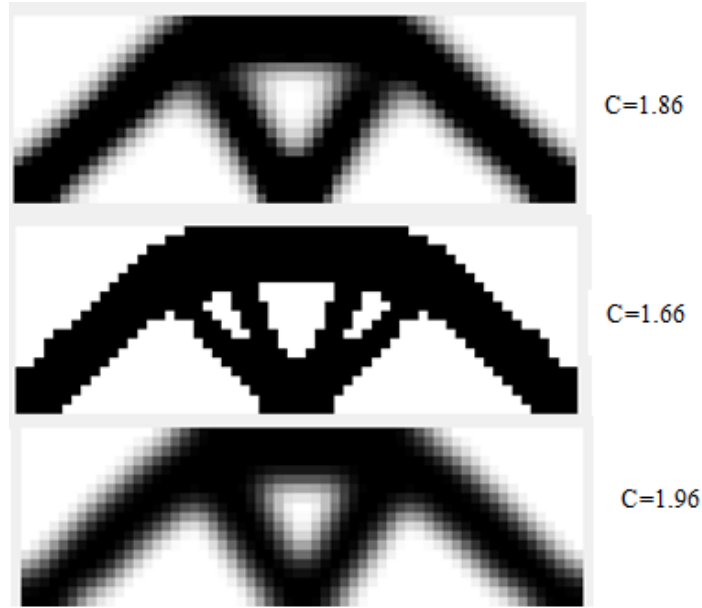
Figure 4.9: Optimum material layout of SSB
