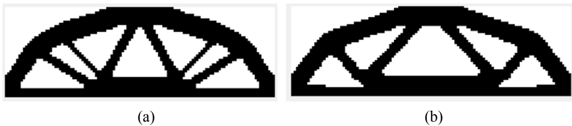
Figure 4.36: Optimum Topology of BESO method (a)4-noded element (b)Higher order elements
