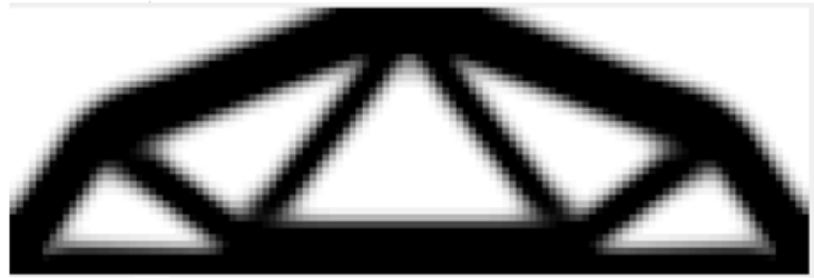
Figure 4.37: Convergence history and Optimum topology of OC method
