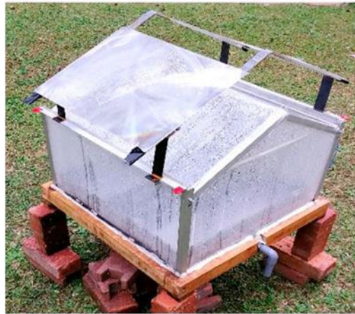
Figure 1.7 Double slope solar still with Fresnel lens (Choong et al. 2020).
