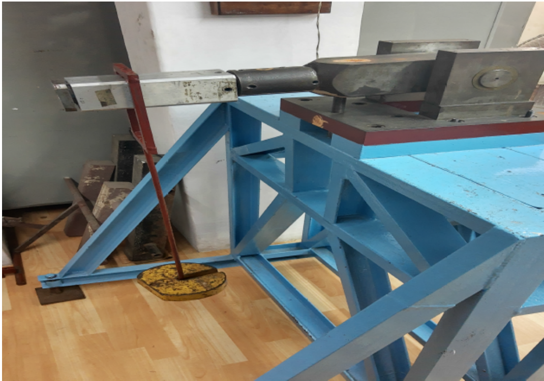
Figure 4.7: Internal balance WT11 under calibration
