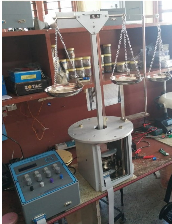
Figure 3.8: Box-type external force balance loaded used a pulley system for calibration-check procedure
