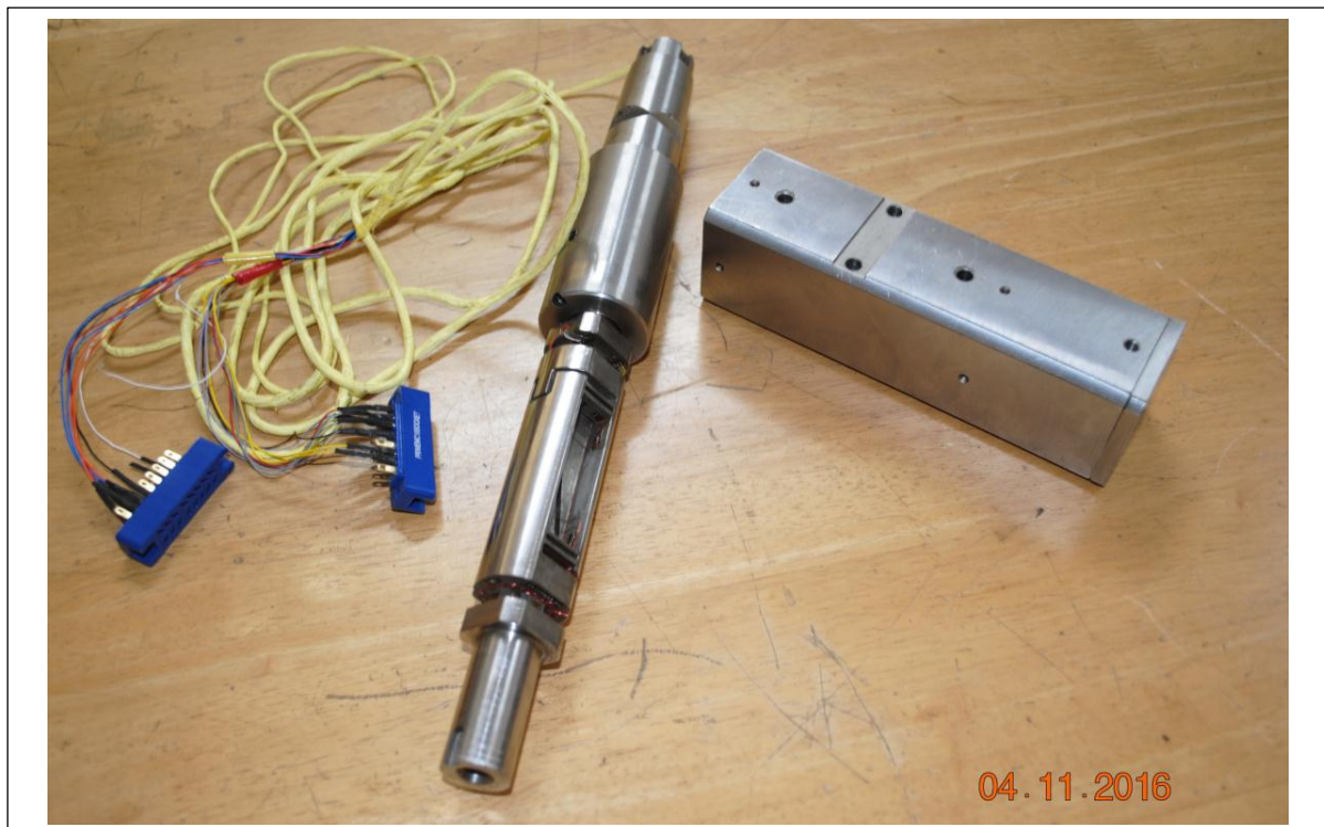
Figure:2 A view of WT11 Balance and calibration body
