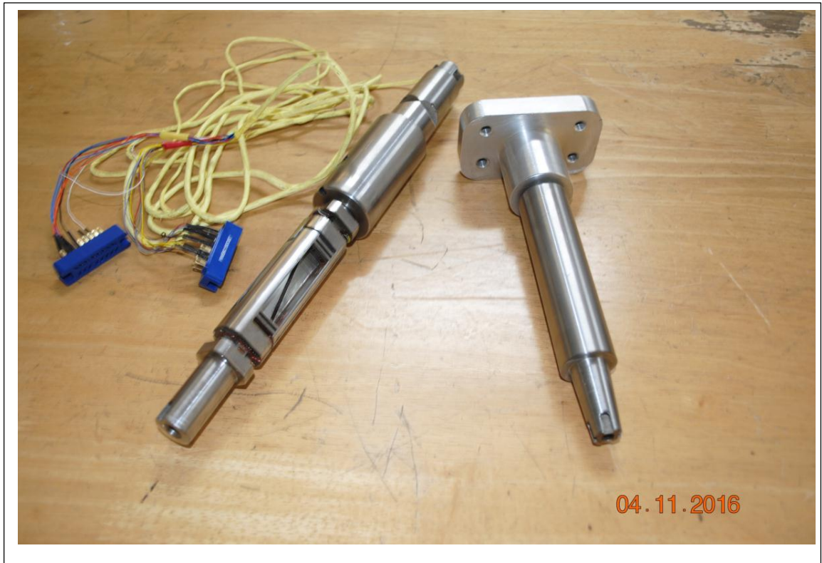
Figure 3: A view of WT11 Balance and Dummy balance with front adapter
