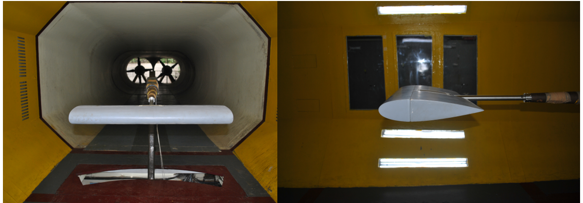
Figure 5.3: Mounting of blade models on tunnel sector arm
