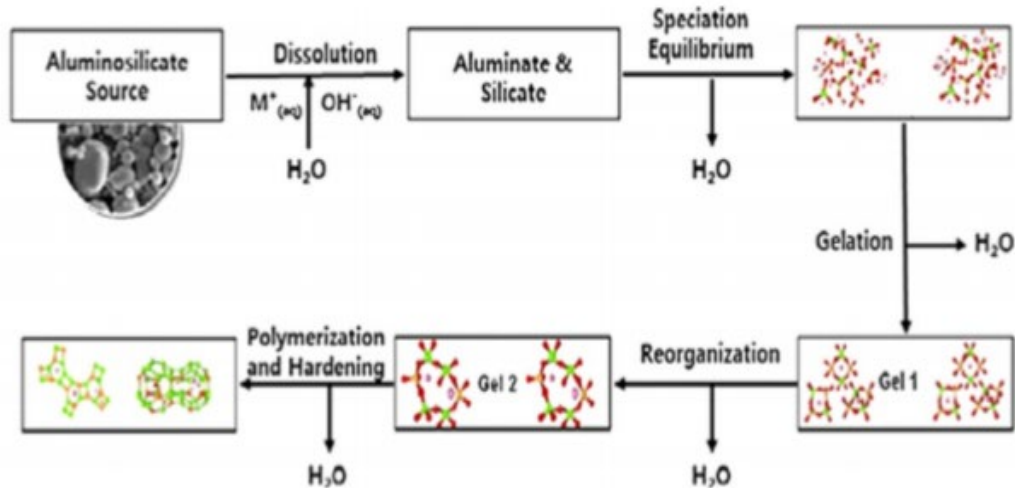
Figure 2.1: Geopolymerization theoretical model representation (Source: Duxson et al. 2007).
