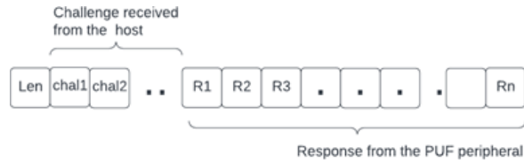
Figure 4.14: Packet format for PUF peripheral
