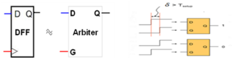
Figure 4.4: Operation of arbiter element
