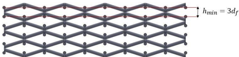
Figure 6.5 Front view of Inline stacking type-b for closely packed scenario (with h_{min} spacing).
