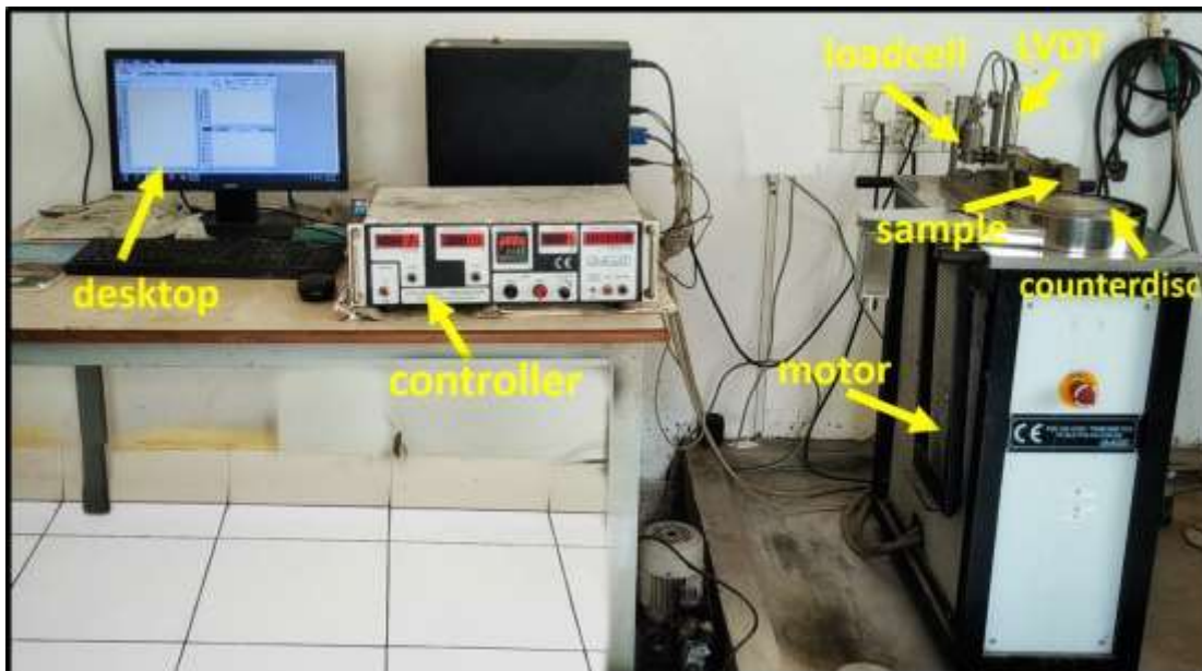
Figure 3.3 Pin-on-disc tribometer used for tribological testing
