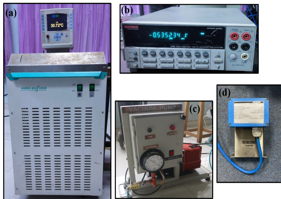
Figure 5.5: Equipment used for test facility (a) Thermostatic bath (b) Data acquisition system (c) Vacuum pump (d) Mass flow meter.
