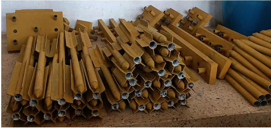
Figure 3.4 Small-scale model piles used in the study
