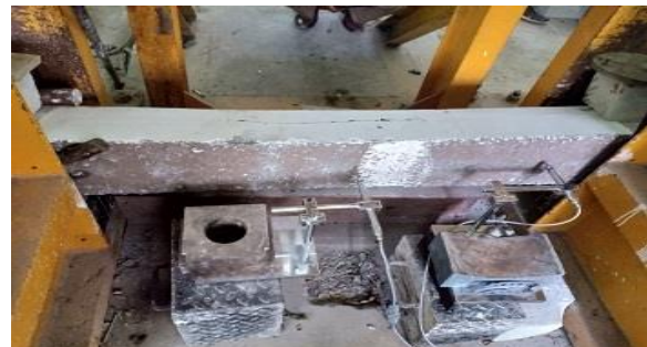
Figure.2 LVDT Instrumentation Used In Experiment
