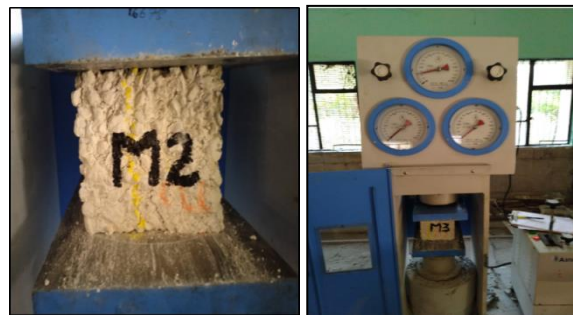
Figure 2: Compression test under progress after total immersion of 56 days
