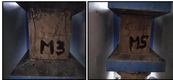
Figure 5: Compression test under progress
