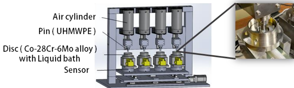
Fig. 1 Pin-on-disc wear testing device
