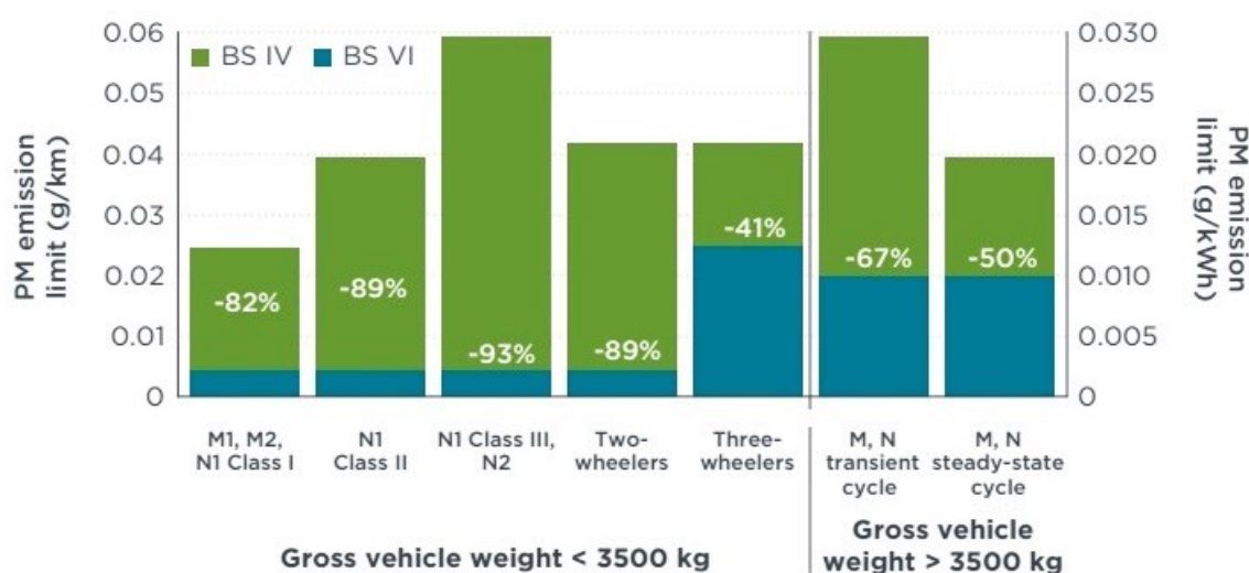
Figure 1.1: Comparison between Bharath Stage IV and VI norms for diesel engines (PM) (IICT 2016).
