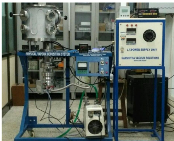
Figure 2.8 VTE system equipped with turbo-molecular pump used for the fabrication of hole- only devices and inorganic-organic p-n junction devices.
