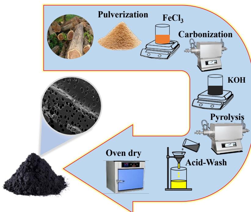
Figure 6.1 Schematic representation of synthesis of Tectona grandis sawdust-derived porous carbon.
