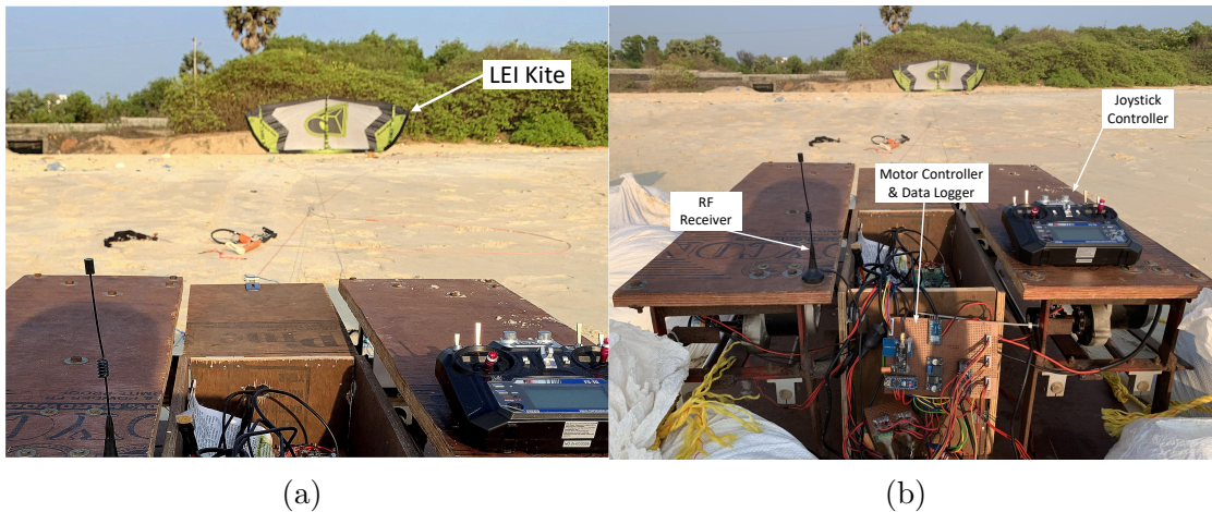
Figure 4.13: (a) Kite used for the field tests (b) Kite steering controller
