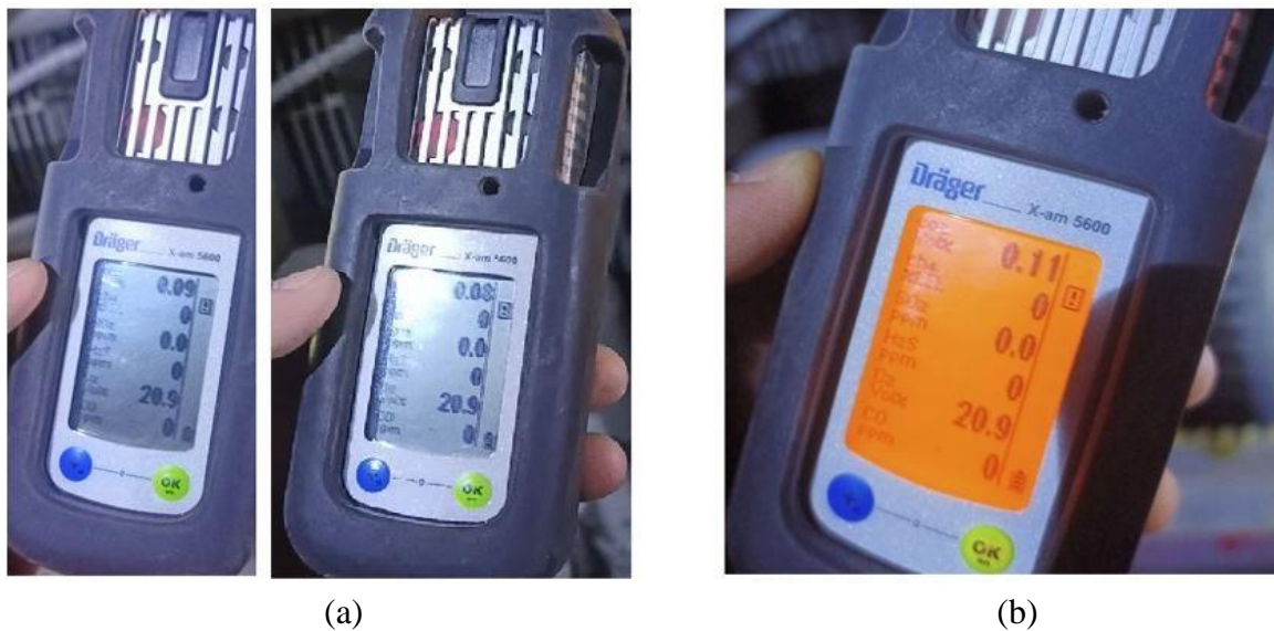
Fig. 5.22 (a & b): Data monitor by the portable multi-gas detector in underground mines ‘A’ and ‘B’
