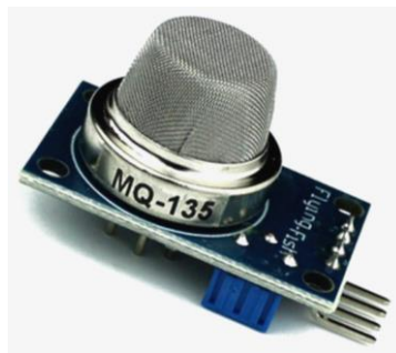
Fig. 3.7 MQ-135 Air Quality Sensor (Sai et al. (2019))
