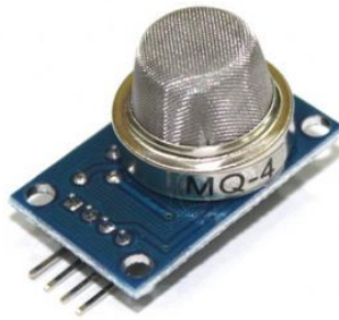
Fig. 3.3 MQ4 - Methane Gas Sensor (Fakra et al. (2020))
