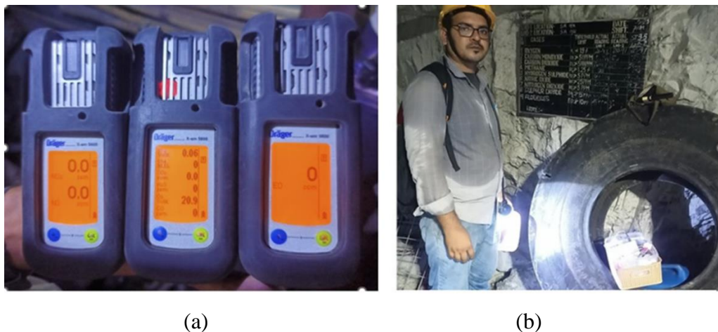
Fig. 2.7 Portable multi-gas detector device and board to display gas parameters (Naik et al. (2024))
