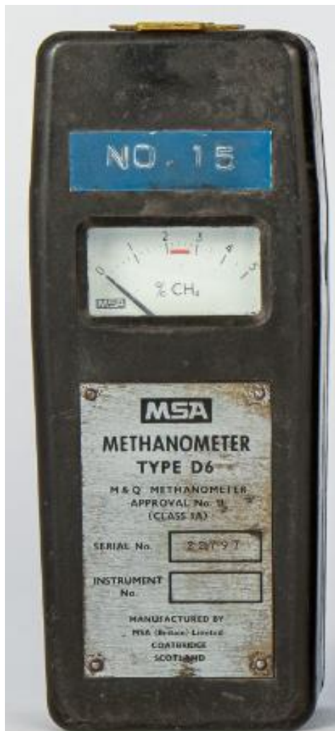
Fig. 2.5 Methanometer used at the Teralba Colliery 1972, (Story Place (2023))
