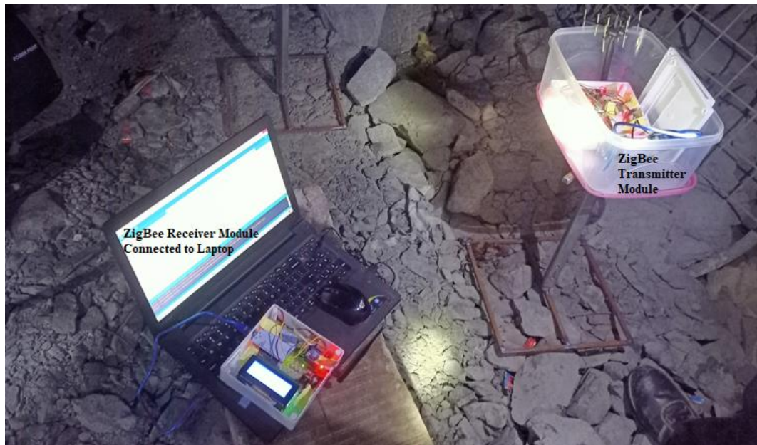
Fig. 5.9 Experimental setup of ZigBee modules in tunnel 26 of Underground Mine ‘B’
