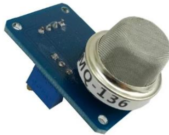
Fig. 3.5 MQ-136 Hydrogen sulfide Sensor (Sanger et al. (2019))
