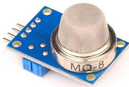
Fig. 3.6 MQ-8 Hydrogen Sensor (Ayub et al. (2020))
