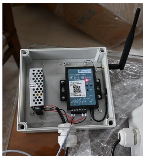
Fig. 4.2 RS485-LN converter device
