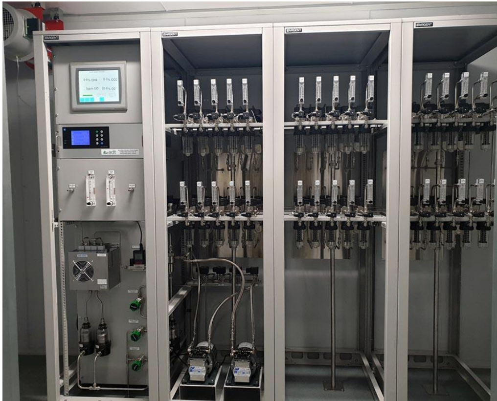
Fig. 2.6 Australian Dynamic Technologies tube bundle systems for underground mines, (Australian Dynamic Technologies (2023))
