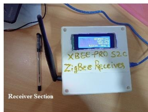
d) ZigBee Module and Sensors placed in a enclosures(Receiver)
