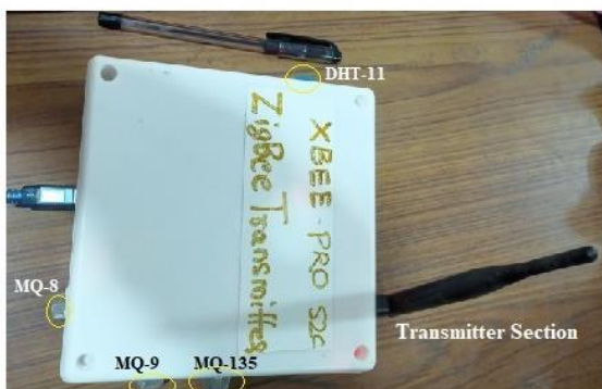
c) ZigBee Module and Sensors placed in a enclosures (Transmitter)
