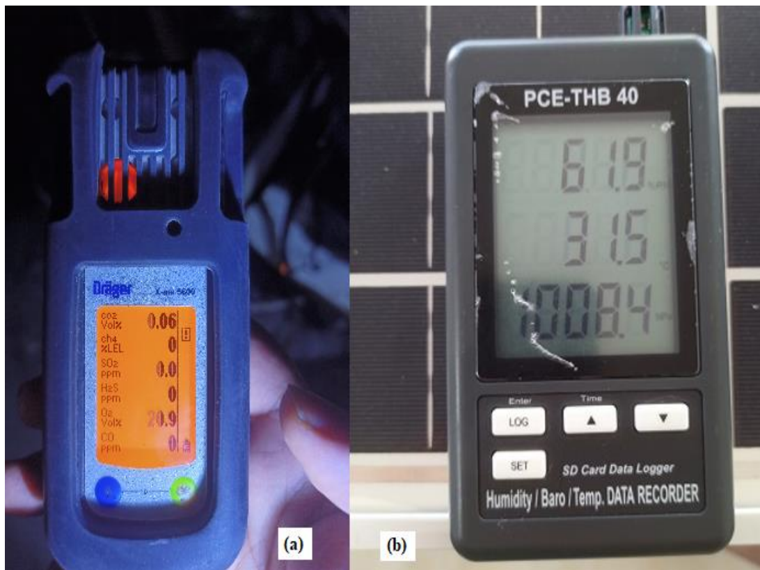
(a) (b) Fig. 5.51 (a &b) Portable Multi Gas Detector Device and Temperature and Humidity Data Recorder
