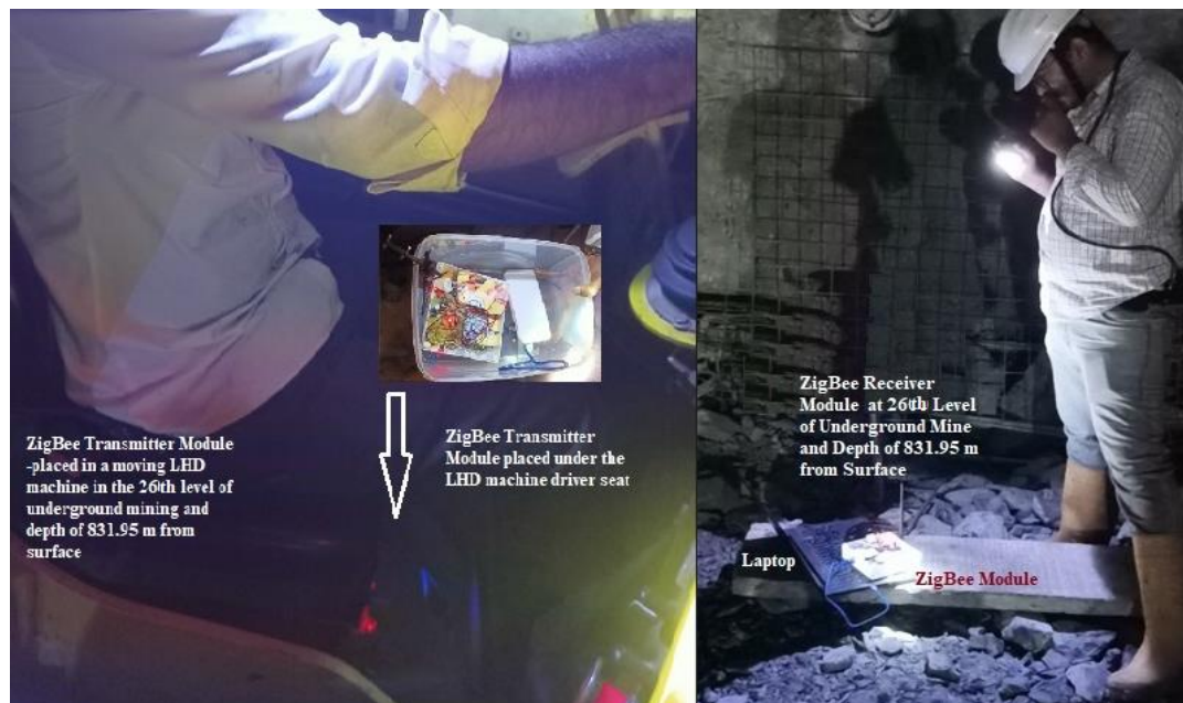
Fig. 5.9 Experimental setup of ZigBee modules in tunnel 26 of Underground Mine ‘B’
