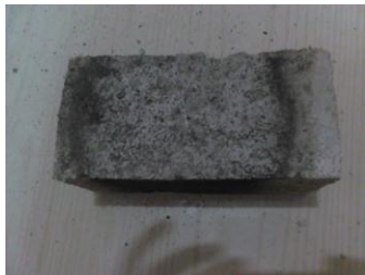
Fig.8 Papercrete brick after fire test
