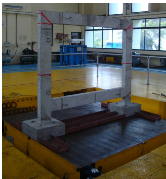
Fig.3 Experimental setup of shake table test of bare frame and masonry infilled frame
