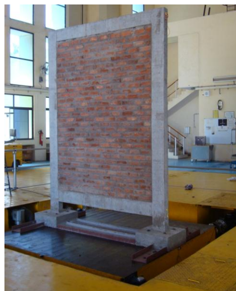
Fig.3 Experimental setup of shake table test of bare frame and masonry infilled frame
